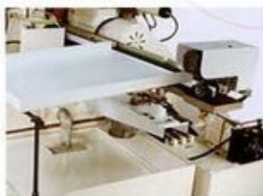
Automatic Unloading Equipment for Thrufeed Grinding (Optional)
